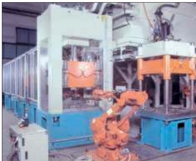
This hydraulic multiple-press system with transfer stations was supplied by Capitol Technologies Inc., allowing an automotive supplier to produce multiple-layer parts in a variety of sizes and geometries.
