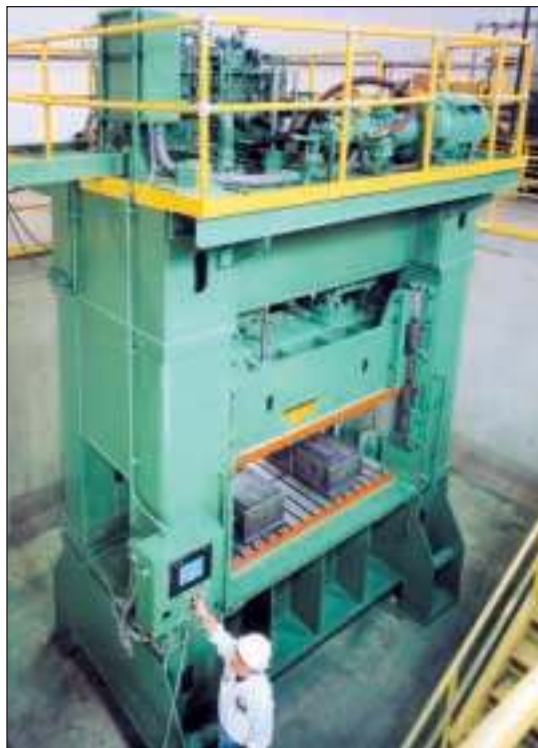
A railcar-equipment maker uses a 750-ton hydraulic press from PH Group Inc. to form 0.75-in. steel plate used to construct tank- and hopper-railcar wheel structures.
