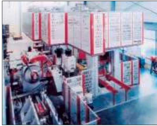
This hydraulic transfer-press line from Schuler Hydrap produces an innovative flywheel component for Mannesmann Sachs AG. Included is a Schuler Automation-supplied coil line. The tooling for the application is shown on preceding page.
