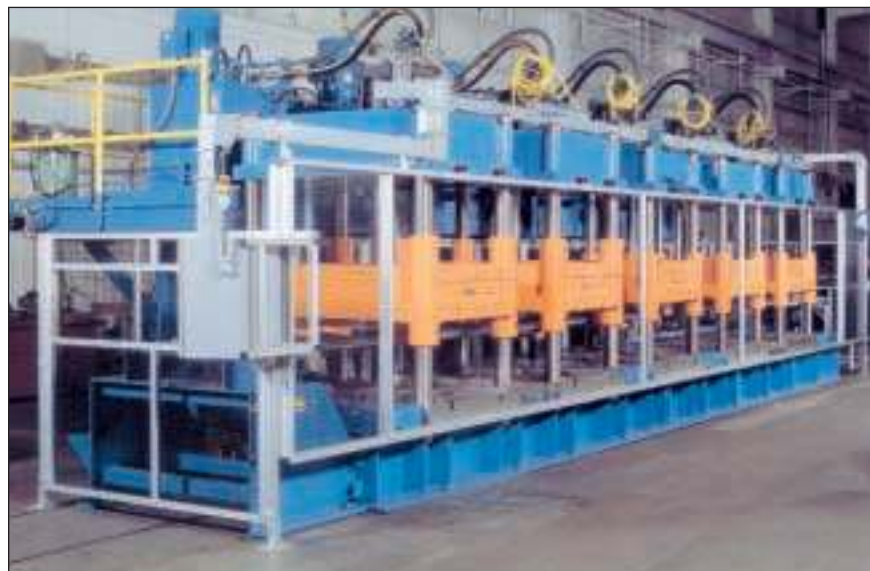
A hydraulic five-press system from Capitol Technologies Inc. helped a manufacturer of steel tool cabinets produce two types of drawers, each with different sizes and depths. The system produces a drawer every 20 sec. while using only two operators.
