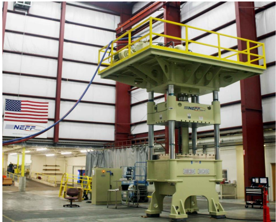
Triple Action 400 ton press with 200 ton cushion.
