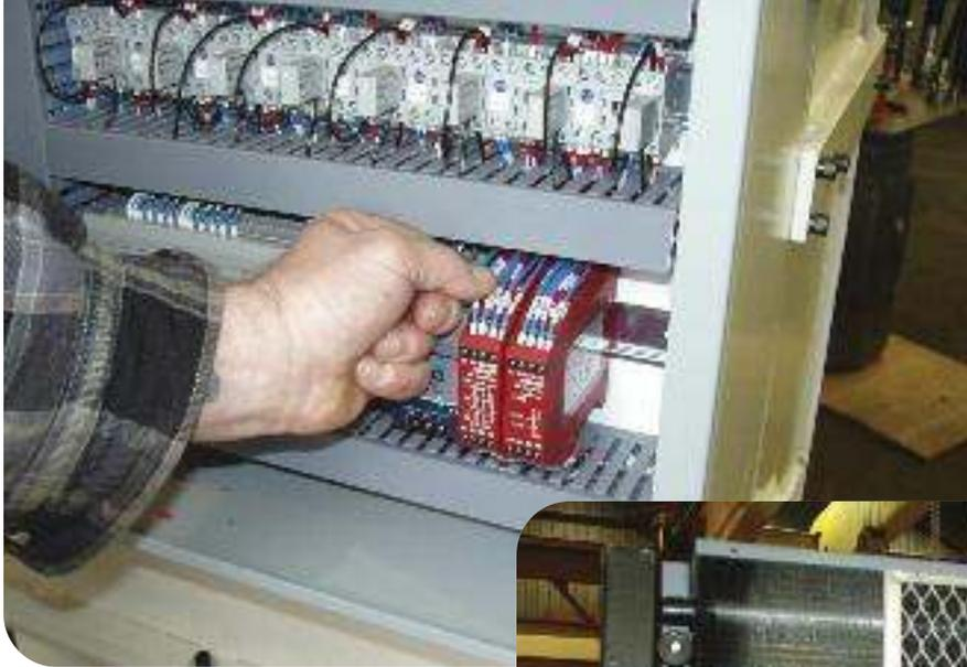
Regularly scheduled preventive maintenance on hydraulic presses should include (top to bottom) checking for loose wiring, inspecting the air filter and greasing the guide rods.
